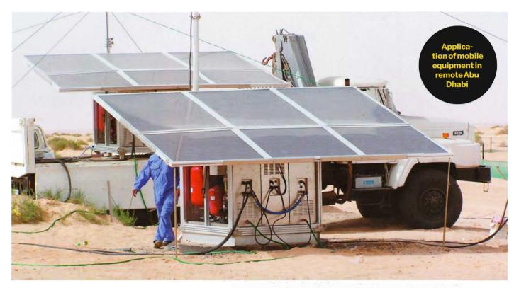
Within the industrial sector, EMRA is positioned to meet specific water requirements through state of the art reverse osmosis portable equipment.'
